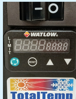
Watlow limit controller
