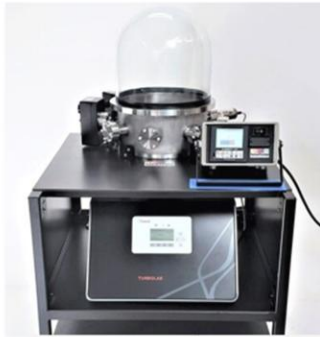
VmSD144-N • Pyrex bell jar • 18" Internal Diameter • 12" or 18" Height • 1 x 10 -6 Torr
