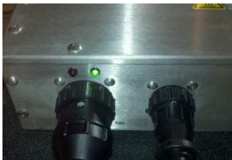
1- Failsafe Working, Normal operation
