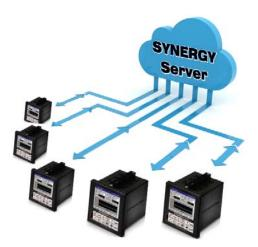
The **Synergy Server** is a web server application designed to virtually unlimited centralized and searchable storage for an unlimited number of Synergy Controllers. Based on Virtual open source LAMP server technology (Linux OS, Apache Web Server, MySQL Database, and PHP scripting platform), the **Synergy Server** provides centralized storage and a simple Web Interface for:
