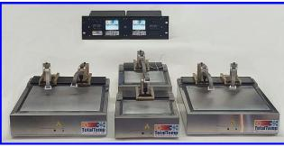
Above the SD144NC-A, SD49NC-A and Dual Synergy Nano Controllers in 19" Rack. HDC was designed to thermally simulate welded RF packages with clamping force.
