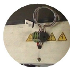
DUT Sensor Terminal Block
