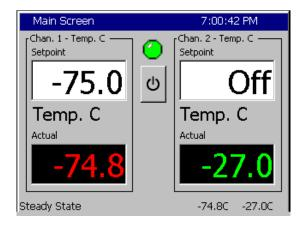
Temperature control is executed using the Channel 1 Setpoint on the upper Left of the screen. The "Actual" temperature reading on the lower left indicates the temperature reading of the controlling temperature sensor embedded in the platform.
