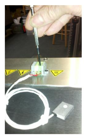
Using a small screwdriver, press down firmly on release spring in the hole above the wire to be inserted or removed.
