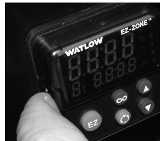
Pull out the tab on each side until you hear it click.
